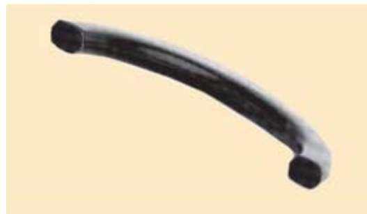
Characteristic compression set - high deformation seen as flattening on all contact surfaces.
