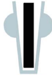
TYPE III ENVELOPE The Envelope Seal construction provides inconsistent results between the two materials. It will also creep, cold flow and leak over time.
