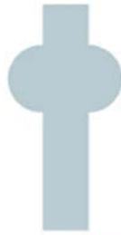
TYPE I A Solid PTFE Type I Seal is guaranteed to fail in SIP conditions. They will creep, cold flow and leak at T Δ
