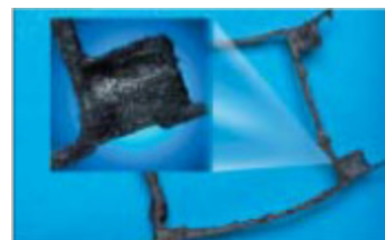
Polymer burn-off of a PREMIER molded part reveals homogeneous fiber dispersion that is key to performance.
