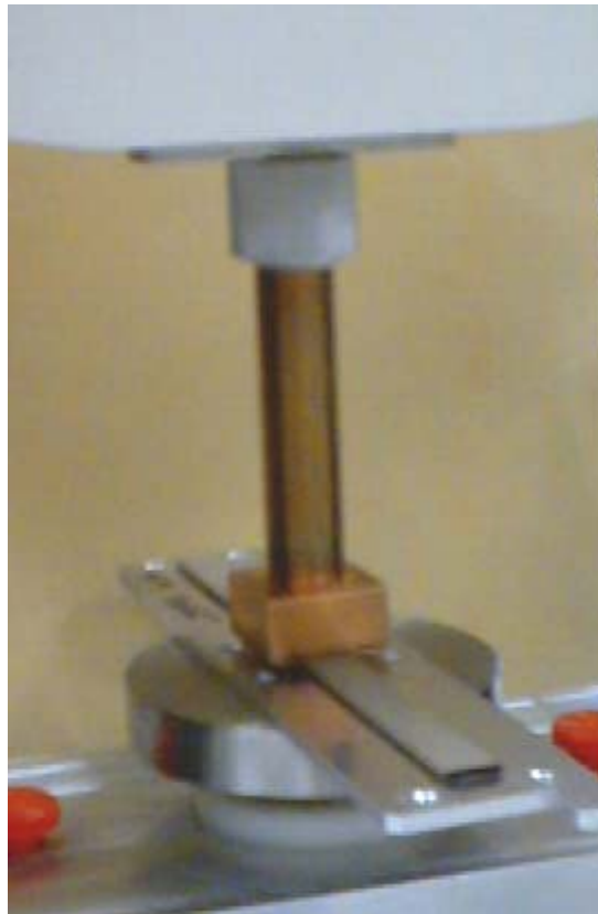
Figure 3. Compression Set Measurement
