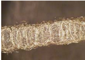
Cross Section showing Multi-planar fiber distribution (10X)
