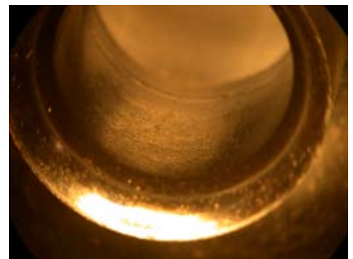
Figure 2 Same sample bore but after heat aging using Parker FKM O-rings with ParkerSlick coating. No coating has bonded into the plastic bore and there are no witness marks from O-ring contact
