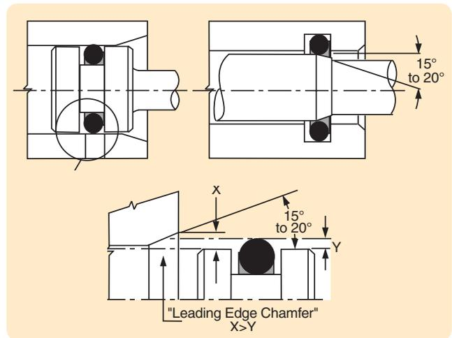
Figure 10-6: Chamfers
