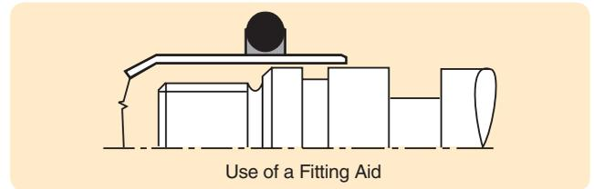
Figure 10-9: Use of a Fitting Aid
