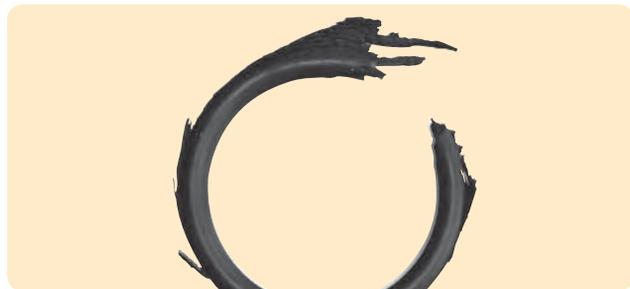
Figure 10-2: Extruded O-Ring
